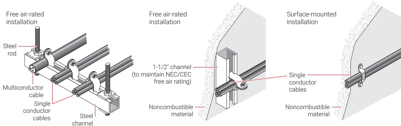
**Fig. 6 MI cable installed on noncombustible surface**
