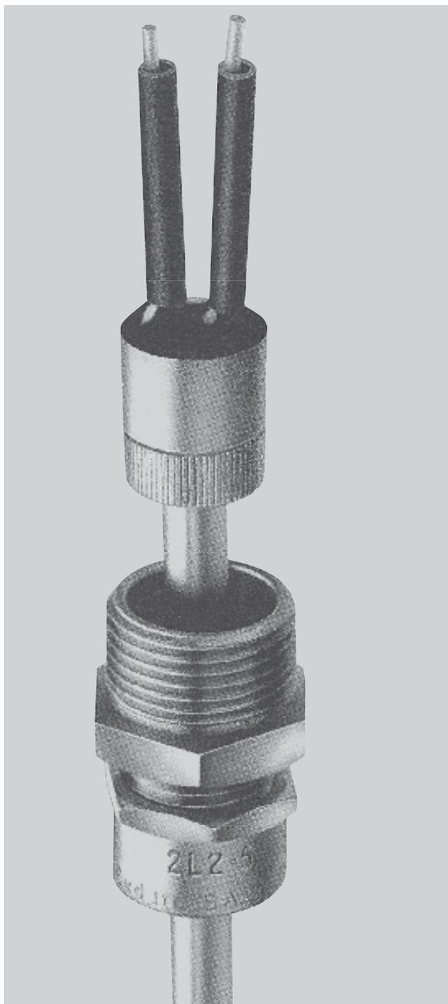
The insulator consists basically of a brass screw-on pot with a glass filling medium and is suitable for use at temperatures between 150°C and 250°C.
