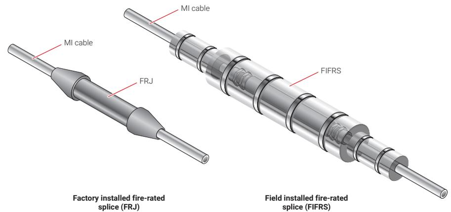
**Fig. 10 Splices for System 1850 MI cable**
