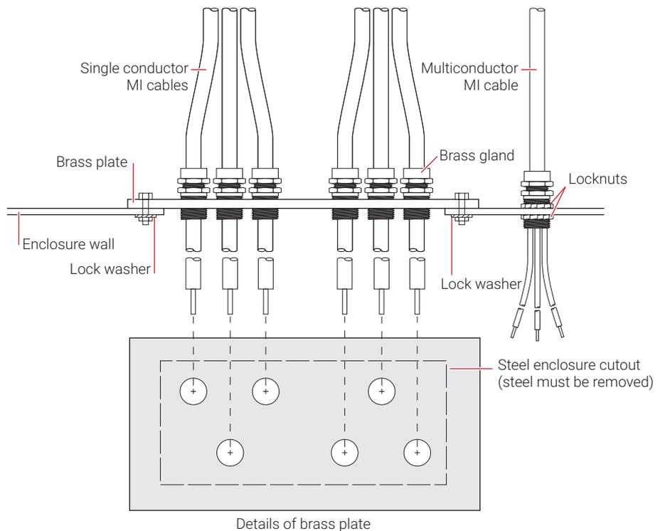
**Fig. 7 Equipment bonding using brass plate**
