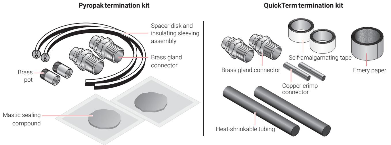
**Fig. 9 Terminations for System 1850 MI cable**
