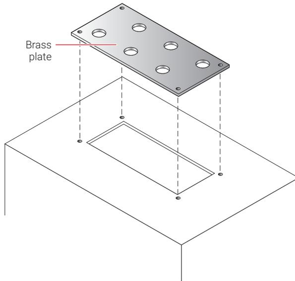
**Fig. 14 Enclosure with cutout and brass plate**
