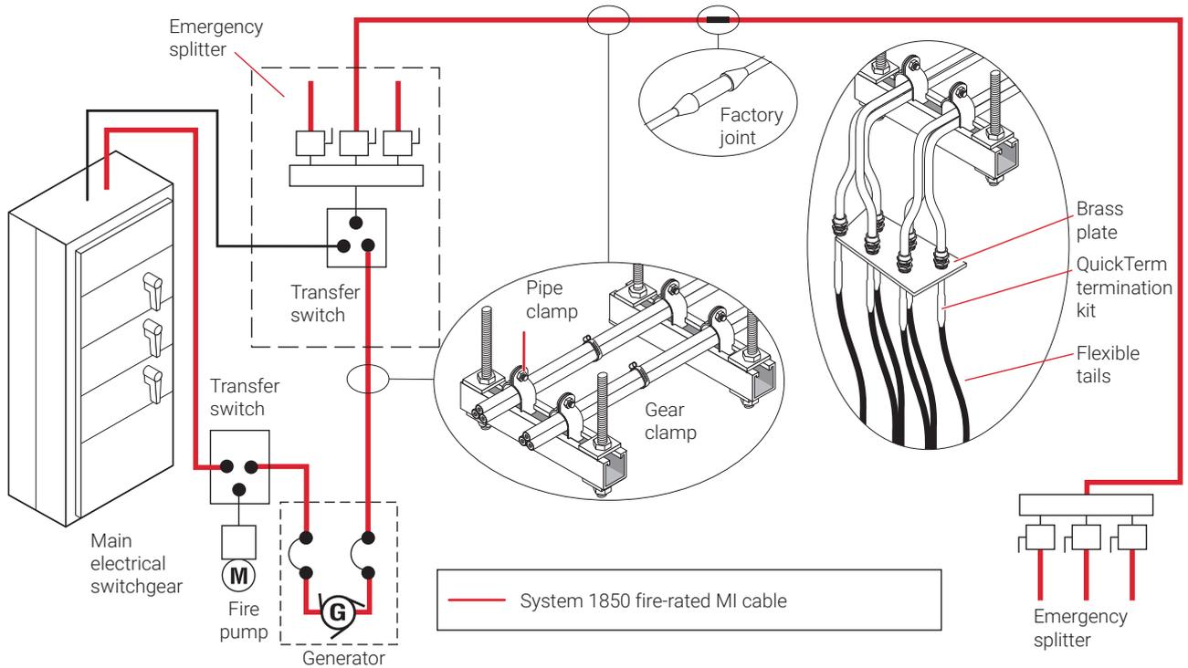
**Fig. 11 Typical System 1850 power circuit system**
