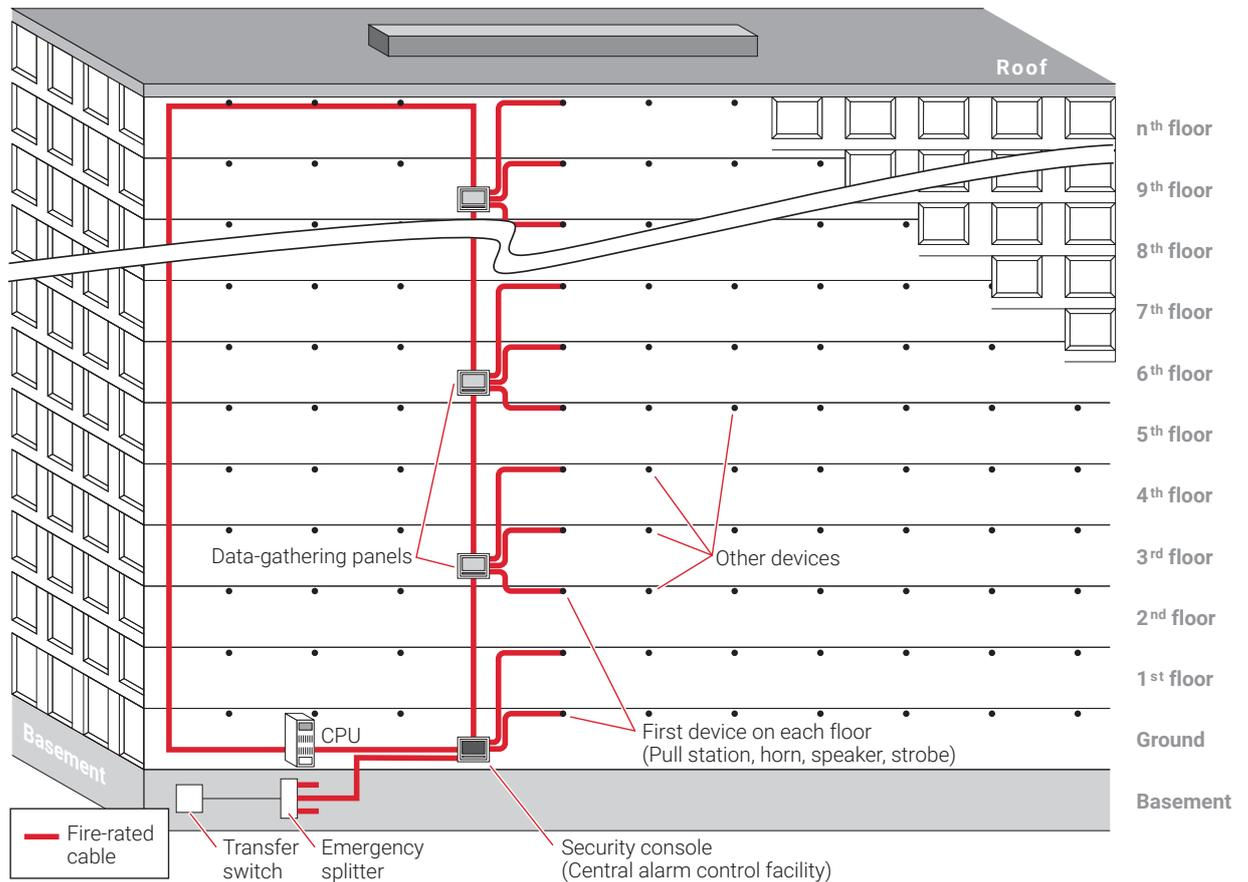
**Fig. 3 Typical fire alarm system**
