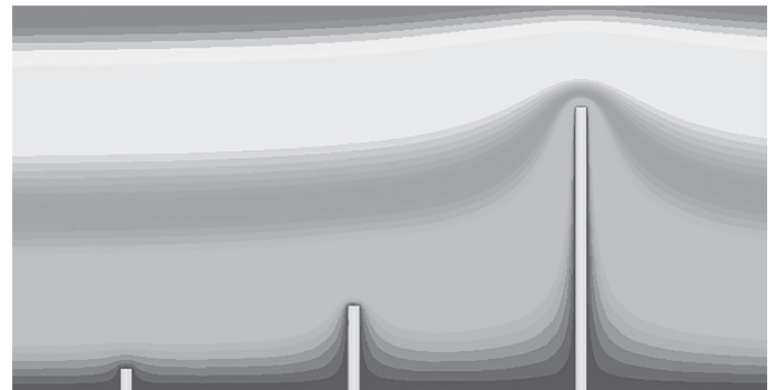
Figure 2. Field intensification, portrayed with lines of equal voltage (equipotential lines), is a function of the height of the object as well as its degree of "sharpness".
